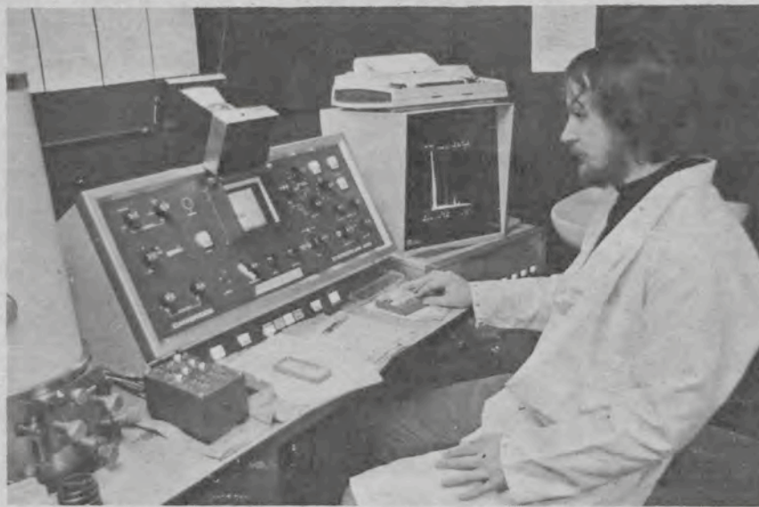
Bill Carey using the scanning electron microscope to check the quality of the materials used for the shuttle experiment. Cosmic Dust penetrations after flight will be examined on this machine at magnifications of up to 50,000.
