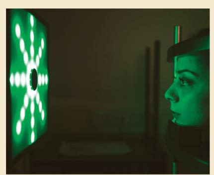
The project has led to the design of a specialist instrument that can capture, in a methodical way, samples of unconstrained iris images from a large number of users. The large database of images has allowed the Kent researchers to develop novel and more robust iris recognition algorithms. The resulting system offers many advantages – for example, the new algorithms allow good recognition performance even when a user's gaze is not optimally aligned with the camera.
