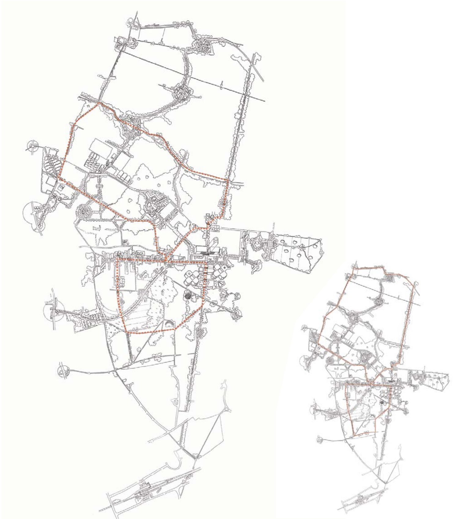
Figure 74: Concept drawing of the proposed 'Circular Cycleway', a 5 kilometre walking, jogging and cycling route around the Campus. Inset: An alternative 7.5 kilometre route
