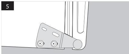
5. Remove the two screws from top bracket and replace on the other side. You will need to first remove the plastic caps from the other side.
