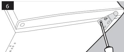
6. Slide the Appliance door back on to the Top hinge, making sure it's the right way up. Screw the bottom hinge into place on the new side. Replace the other foot on the other side. Replace the plastic covering by clicking back into position on the door hinge.
