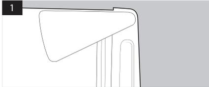
1. Remove the plastic covering from the bottom door hinge.
