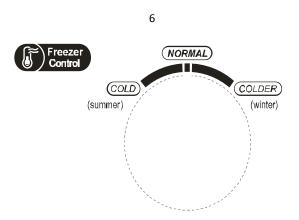
The freezing temperature is relatively low in "COLDER" position, while the freezing temperature is relatively high in "COLD" position, thus, "NORMAL" position is generally used.
