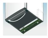
6. IReplace the bottom hinge to the other side then fix it with screws.
