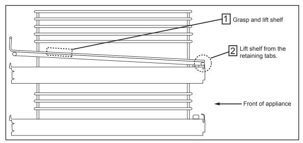
Before removing the shelves completely, please make sure that the shelf is unclipped from the retaining tabs.
